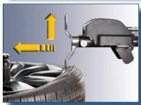
MANUAL ROTATION OF THE TOOL ALLOWS THE OPERATOR TO SWITCH QUICKLY AND EASILY FROM DEMOUNTING TO MOUNTING MODE
