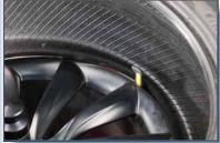
☐ The mounting phase of the second bead is completed by **using the bead breaker disc** and the turntable rotation at the same time, while in case of either low-profile tyres or RFT tyres, a bead pressing tool shall be used to ensure that the tyre remains on the rim channel.
