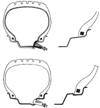
**II - Rim (Wheel).** The wheel is the rigid metal part which connects the vehicle hub to the tyre, on a fixed but non-permanent basis.
