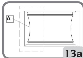
**High performance wheels (asymmetric curvature) - Fig. 13B** some European wheels have rims with a very pronounced curvature C, except in the area of the valve hole A where the curvature is less pronounced B. On these wheels the bead must first be broken in the area of the valve hole, on both the top and bottom sides.
