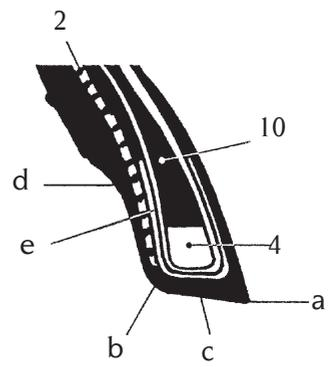
is the outer part of the bead. The base (c) is the area resting against the rim. The groove (d) is the concave part against which the rim shoulder rests.
